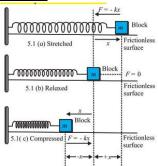
The force in the spring is always directed to the mean position and is responsible to bring the block back. This restoring force is proportional to the displacement from the mean position.
